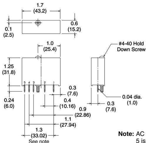
**Note:** AC and DC input versions only; pin 5 is not present on output modules.
